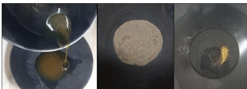
Figure 2 Procedure for separating gold from other sediments using O. pyramidale extract.
