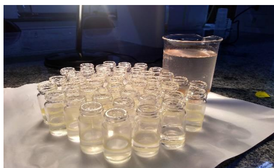
Figure 2 Illustration of biosurfactants toxicity testing (0.3 g/L, 0.6 g/L, and 1.2 g/L) using microcrustacean larvae after a 24-hour incubation period.
