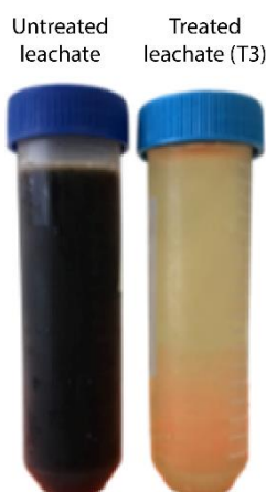
Figure 2 Visual reduction of color considering the untreated leachate and the best condition (T3).
