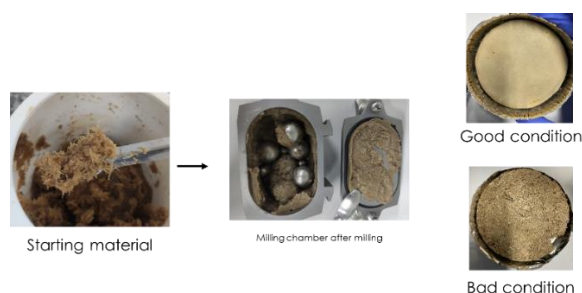
Figure 2: Visual depiction of satisfactory and unsatisfactory milling conditions.
