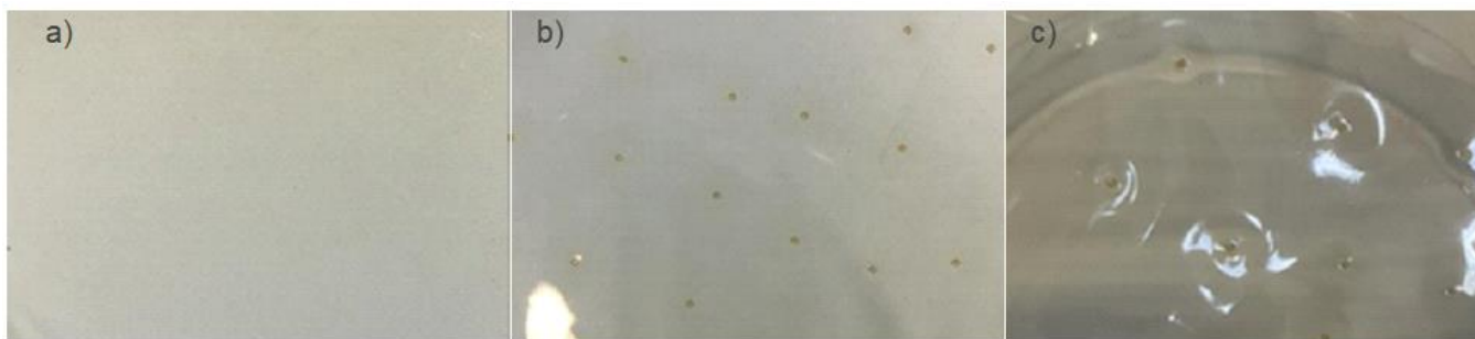
Figure 1 Typical visual aspect of films analyzed by visual inspection: a) Alginate film without particles; b) Film with drug-free particles; c) Film with particles containing Keto.
